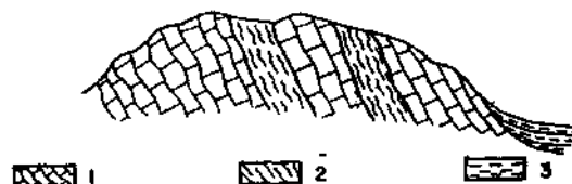
Fig. 5 - Schematic drawing showing the contact between crystalline limestones and schists on the hill east of Akçaköy
