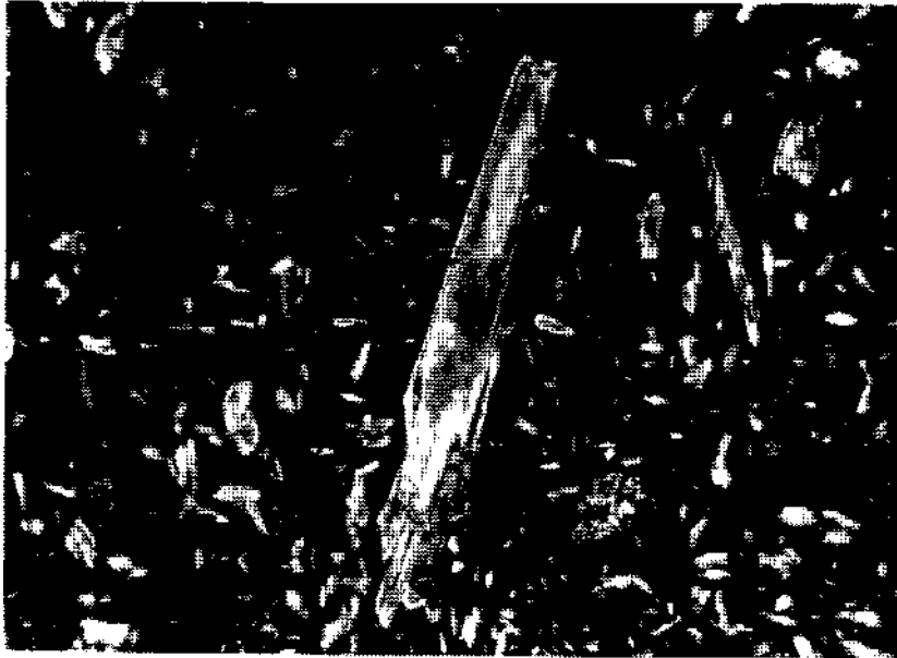
Photo 15 - Hydroboracite heated to 250°C (100 ×, + N).
