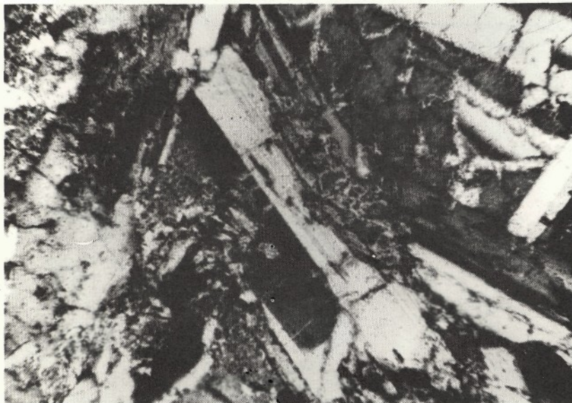
Fig. 14.- Diabase-basalt, plagioclases and augite crystals, in ophitic intergrowth. N +; 140 x. Photo taken by: D. Pestic.
