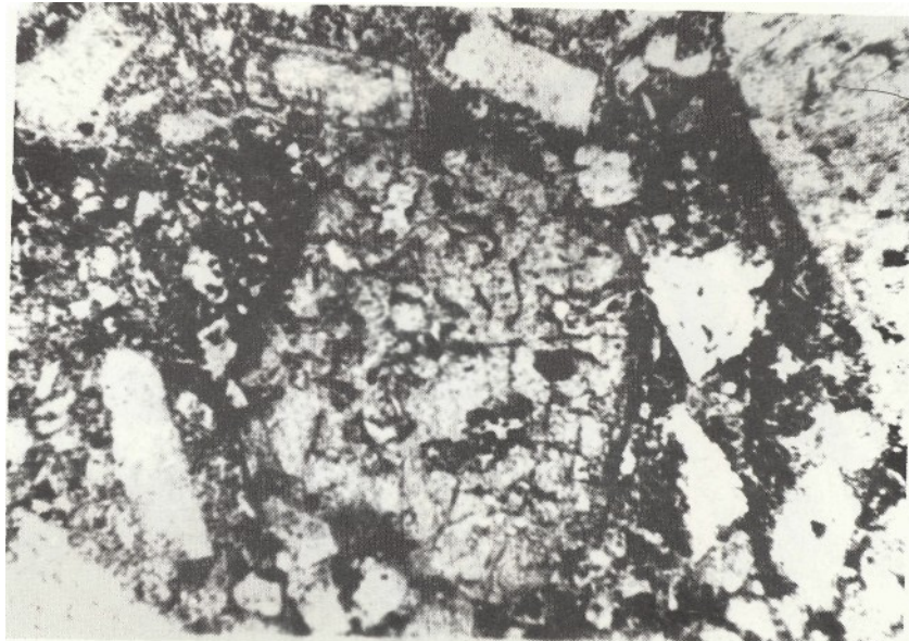
Fig. 12 - Augite, andesite: plagioclase and augite phenocrysts. N//; 140 \times . Photo taken by: D. Pesic.
