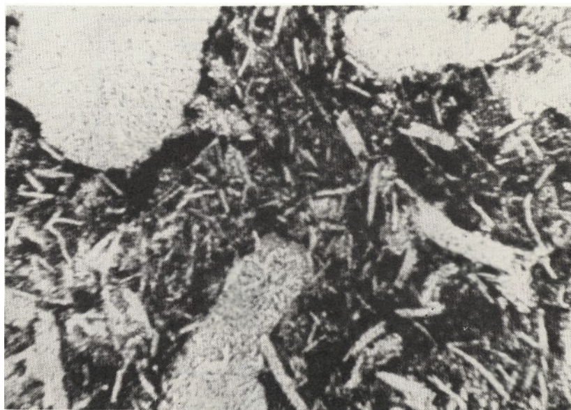
Fig. 4 - Basalt, amygdaloidal, albite with much opaque mineral powder. N//; 140 ×. Photo taken by: D. Pesic.
