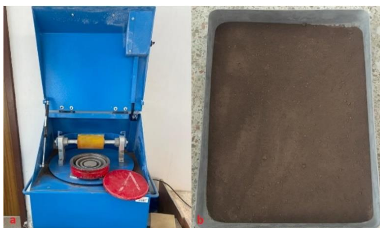
Figure 2. Ring mill used in the experiment (a) and PP (b)
