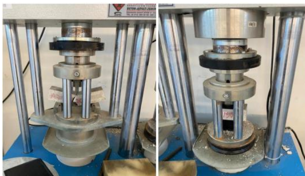
Figure 4. Flexural strength tests (three-point) and compressive strengths test
