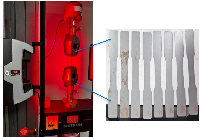
Figure 6. Tensile strength test apparatus and specimens according to JIS Z 2241 0^\circ , 45^\circ , 90^\circ XX1, XX2.
