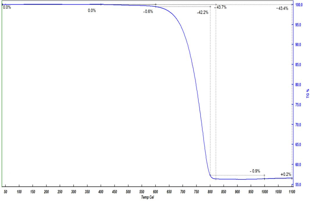
Figure 5. The Result of TG Analysis (% Loss of Weight)
