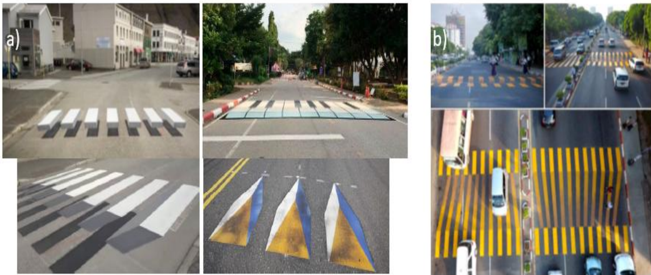
Figure 1. 3D pedestrian crossings in different designs: a) the impression of a high platform [7], [15], [20] b) the impression of a downward slope [9]
