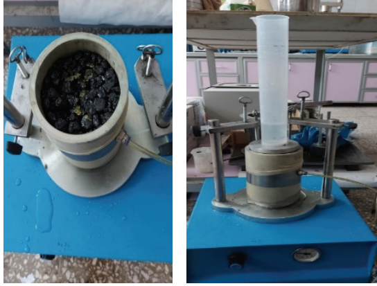
Fig.11 - Placement of samples in the permeability device
