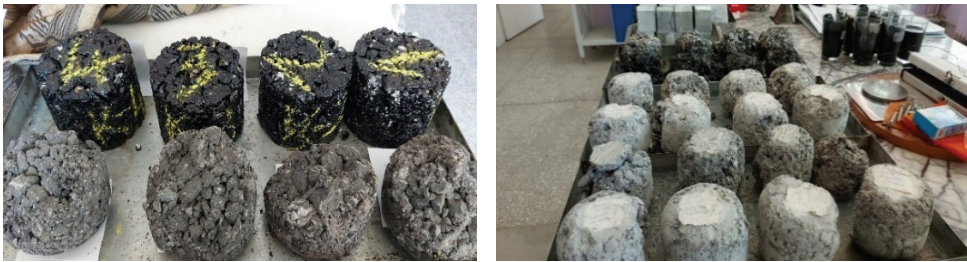
Fig.9 - Mixture specimens after the Cantabro test
