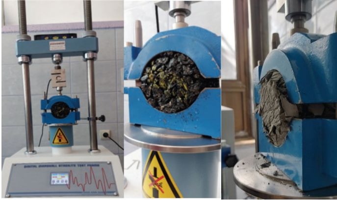
Fig.8 - Placement of Porous Asphalt and Semi-Rigid mixture samples in the Marshall device
