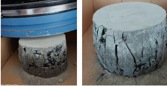
Fig. 12 - Placement of the semi-rigid mixture specimen in the concrete compression machine and the specimen after the test
