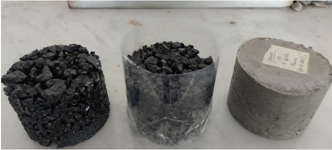
Fig 3 - The preparation of semi-rigid mix samples.
