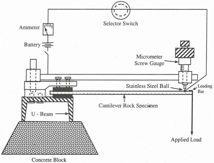
Figure 1. Deflection Measurement with Electrical Circuit System. <sup>6</sup>
