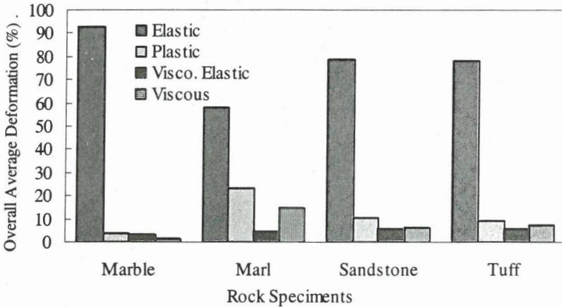
**Figure 2.** Graph of Overall Average Deformations for Various Components of Deformations.
