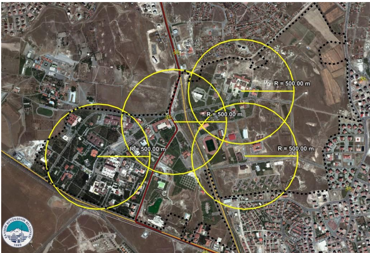
Figure 8. Determination of service areas by radius (Source: Prepared using the Kayseri Metropolitan Municipality CitySurf application)
