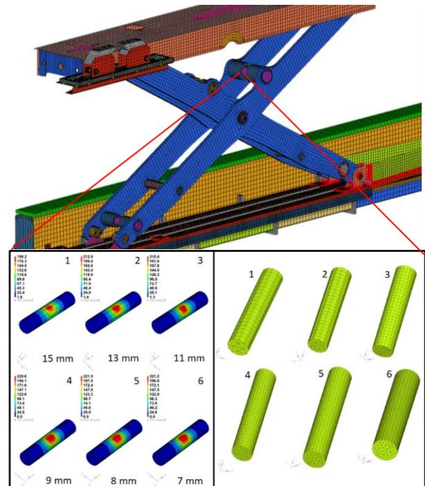
Figure 3. Mesh optimization for the critical component.
