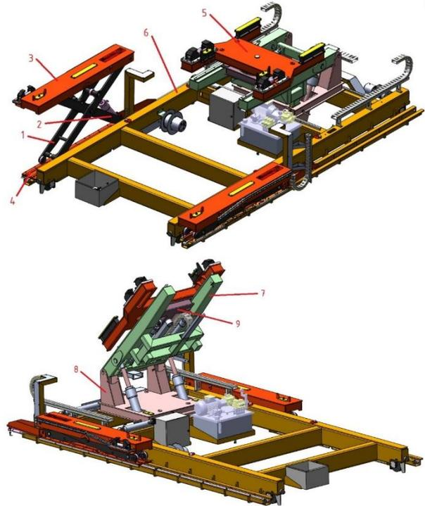
1; outer scissors, 2; inner scissors, 3; scissor lift upper platform, 4; scissor lift lower platform, 5; chassis bracing upper platform, 6; lower chassis, 7; vertical positioner, 8; horizontal positioner, 9; rotation group.
