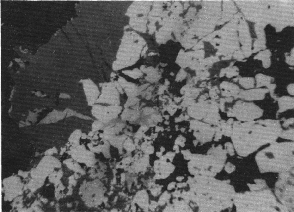
Fig. 8 - Infillings of tetrahedrite (dark gray) between pyrite grains (white). Siderite (black). Polished Section, //N, 32 X, in immersion oil.
