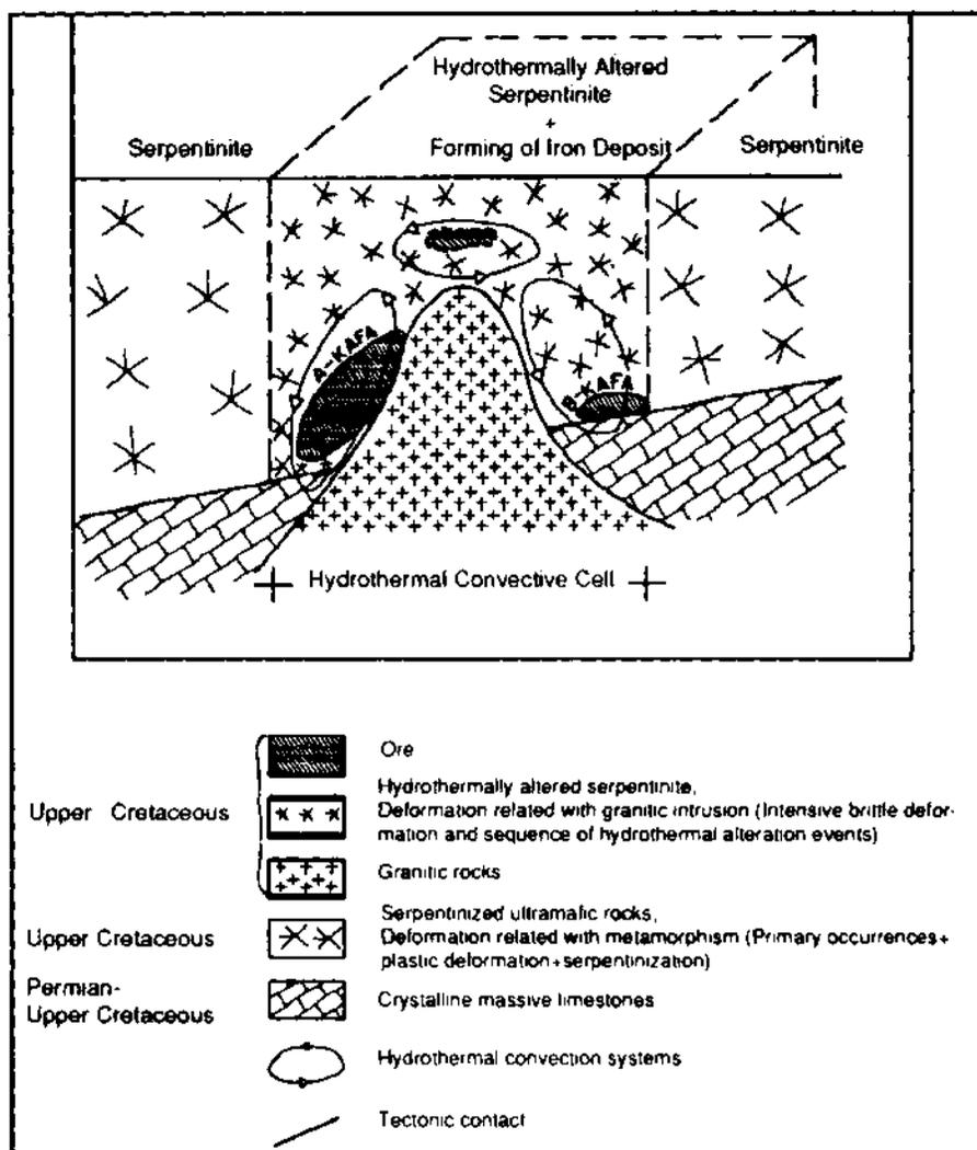
Fig. 3- Schematized formation model of Divriği A- and B- Kafa iron deposits (non scaled).
