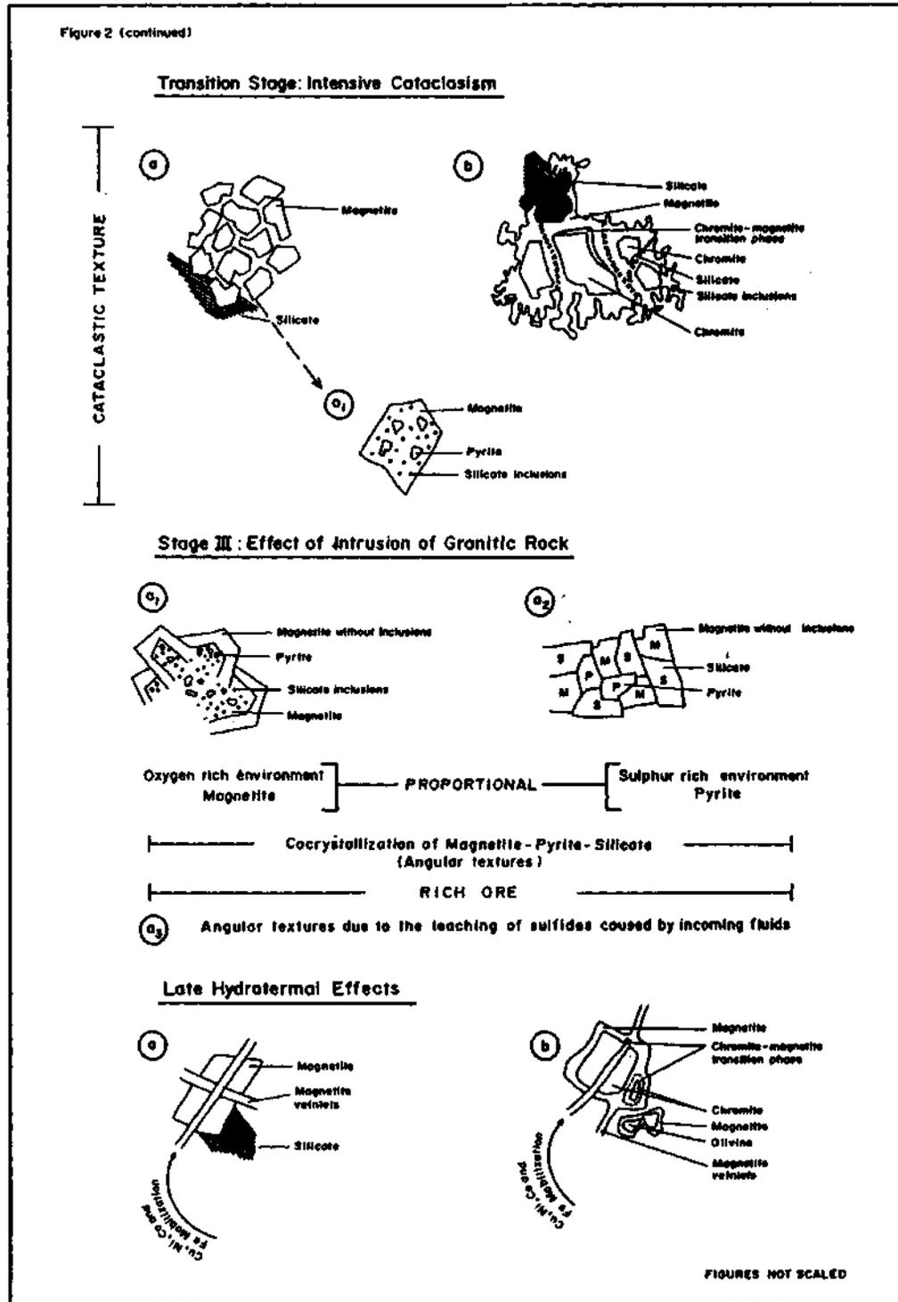
Fig. 2- Textural characteristics of different mineralization stages from older to younger (Stage II and Transition Stage silicate minerals are mainly serpentinite minerals like chrysotile, antigorite etc. Stage III silicate minerals are mainly chlorite, biotite, phlogopite and/or muscovite. No cataclasis have been observed on mica minerals. Very fine-grained, anisotropic silicate and/or carbonate minerals are also observed in the Transition Stage a).
