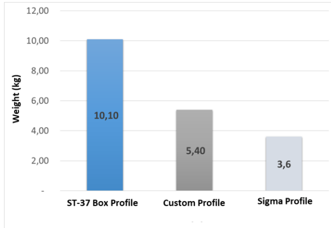
Figure 3. Weight comparison of profile types (770 × 40 × 120 mm).
