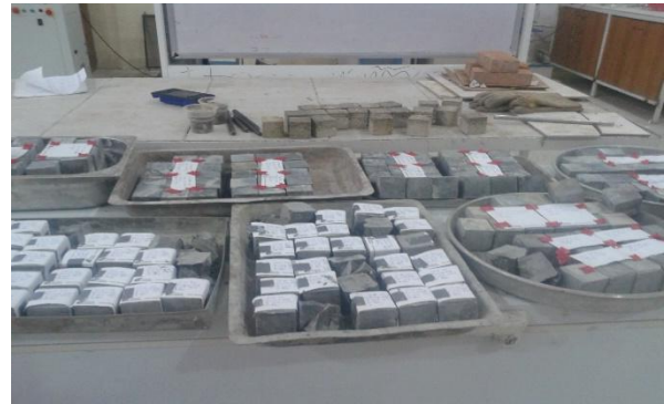
Figure 10. Samples to be broken in the concrete press after leaving the autoclave.
