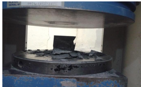
Figure 11. Sample broken in the concrete press.
