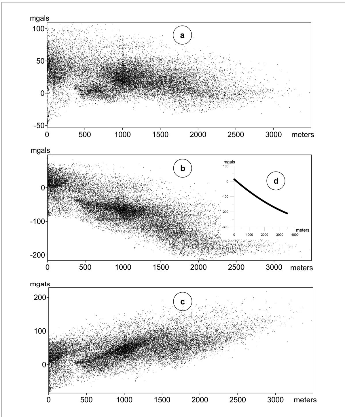
Figure 6- Behaviour of the isostasy (a), Bouguer (b) and free air anomalies (c) by altitude changes; The polynomial relation of second degree between Bouguer and altitude (d).
