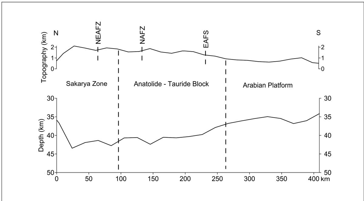
Figure 12- The vertical section of the profile 4 in N-S direction showing topography and crustal thickness.
