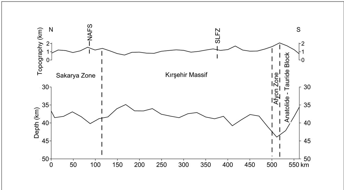
Figure 11- The vertical section of the profile 3 in N-S direction showing topography and crustal thickness.
