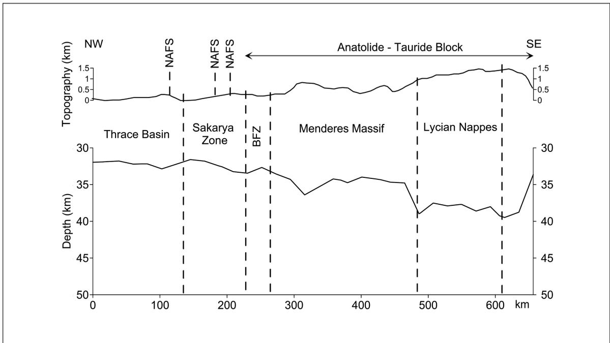
Figure 9- The vertical section of the profile 1 in NW-SE direction showing topography and crustal thickness.
