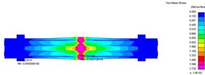
Figure 9. Von Mises Stress for MAT1 Material
