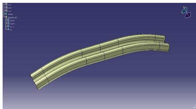
Figure 1. Design of Bumper from Catia V5
