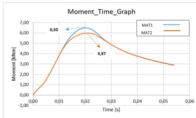
Figure 6. Moment-Time Graph After Simulation
