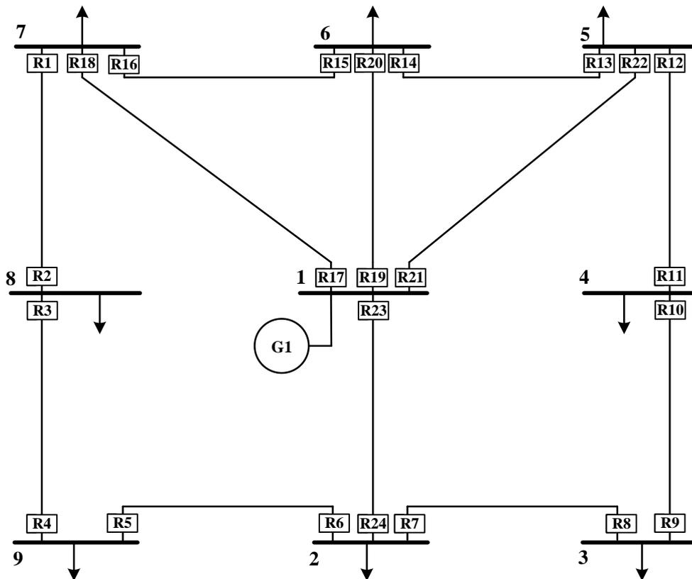
**Figure 2.** Single-line diagram of the IEEE 9-bus test system (IEEE 9-bara test sistemi tek hat şeması)
