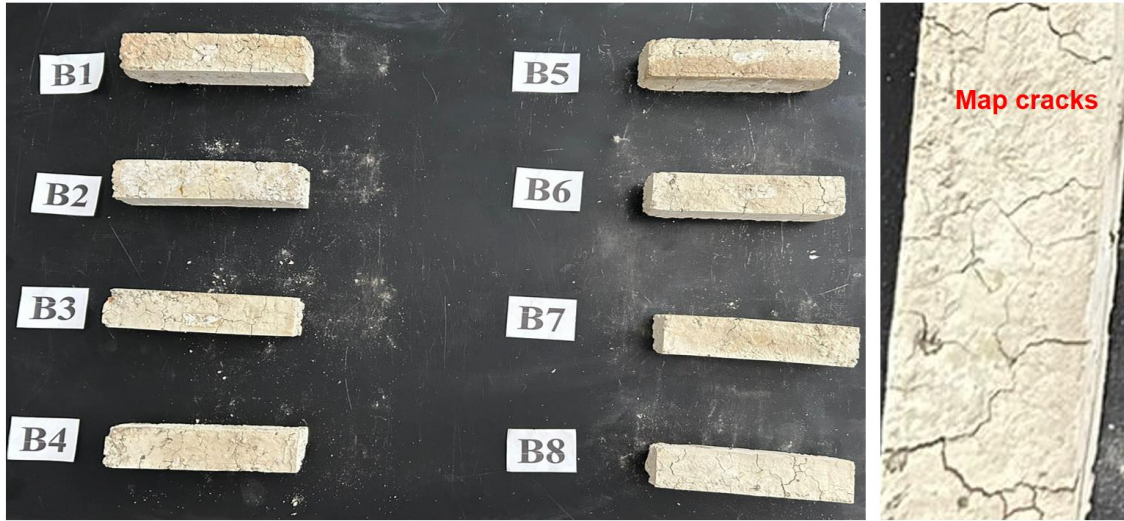
Figure 6. Foam concretes containing CS exposed to 900°C (900°C'ye maruz kalan CS içeren köpük betonlar)
