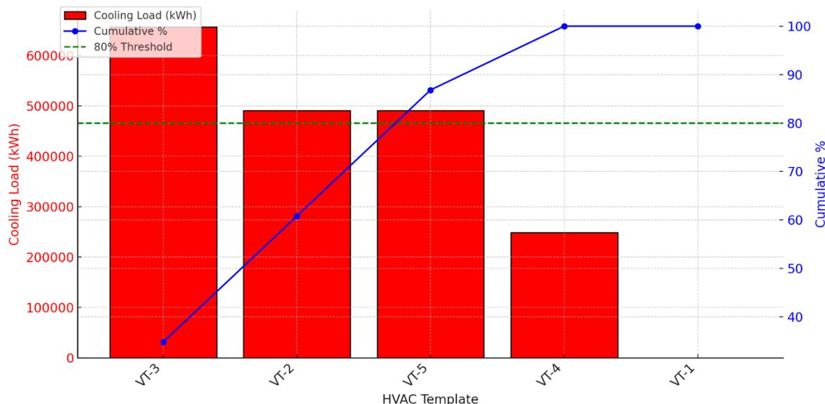
**Figure 9.** Comparison of cooling loads for five HVAC systems under a 30% window opening ratio and no shading (SE-1) condition, with cumulative impacts analyzed using Pareto analysis.
