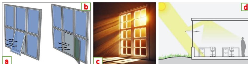
**Figure 1** (a) Natural ventilation in the current window system, (b) Enhancement of natural ventilation, (c) The impact of solar radiation on the indoor environment, (d) Schematic representation of solar control systems.
