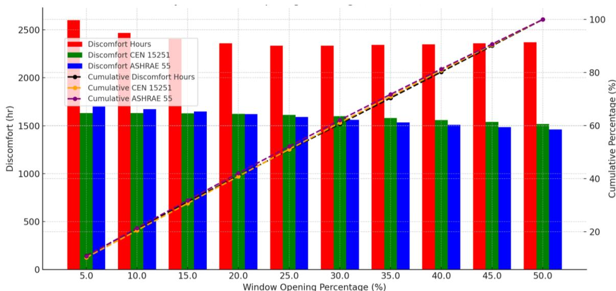
**Figure 6.** Impact of Window Opening Ratios on Discomfort Criteria under SE-1 (No Shading) and VT-1 (Natural Ventilation - No Heating/Cooling) Scenarios"
