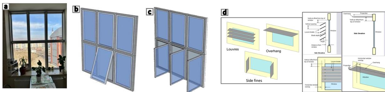
**Figure 4(a)** Current window system with a 5% opening ratio representing the baseline scenario, **(b)** Existing window structure with six casements, including two vertical and one horizontal section, **(c)** Maximum window opening scenario with 50% opening, where the three lower
