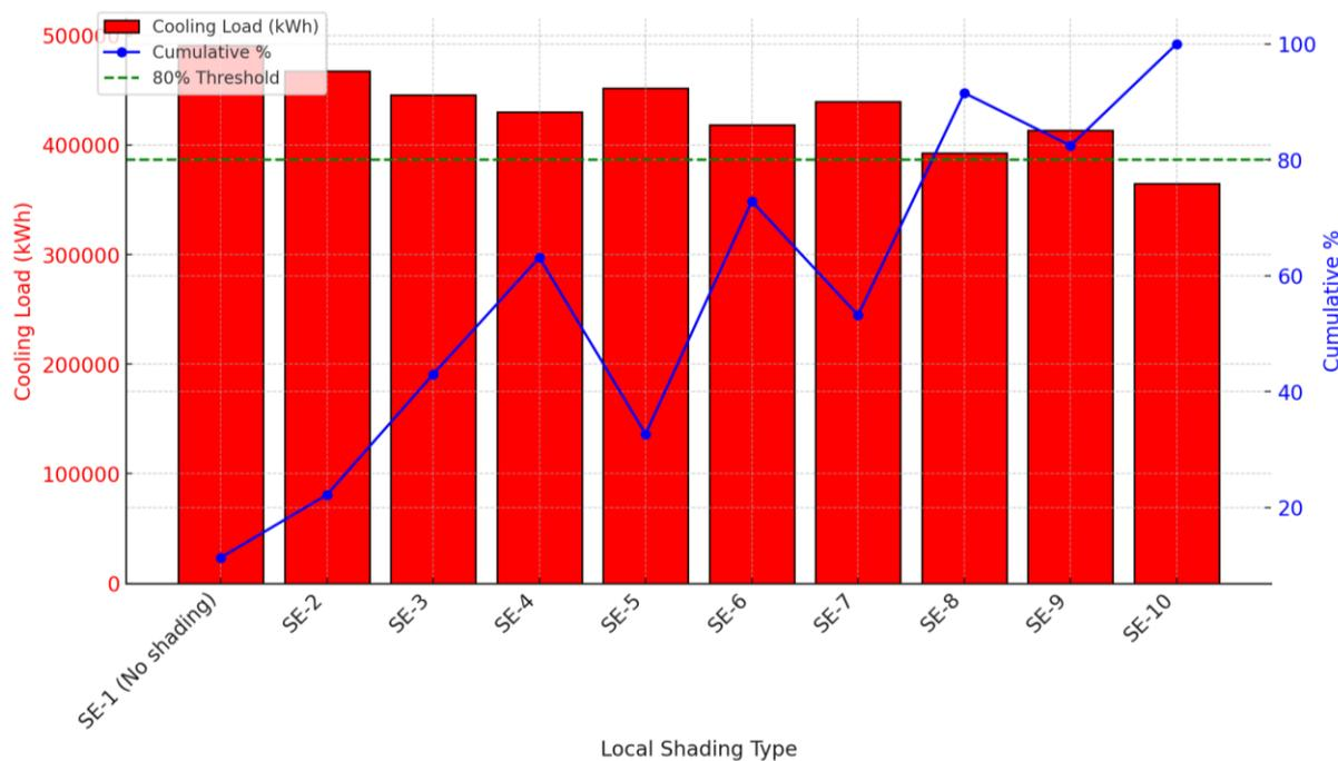
**Figure 10.** Comparison of cooling loads for different shading element types under the VT-2 HVAC system and a 30% window opening ratio, with cumulative impacts analyzed using Pareto analysis.
