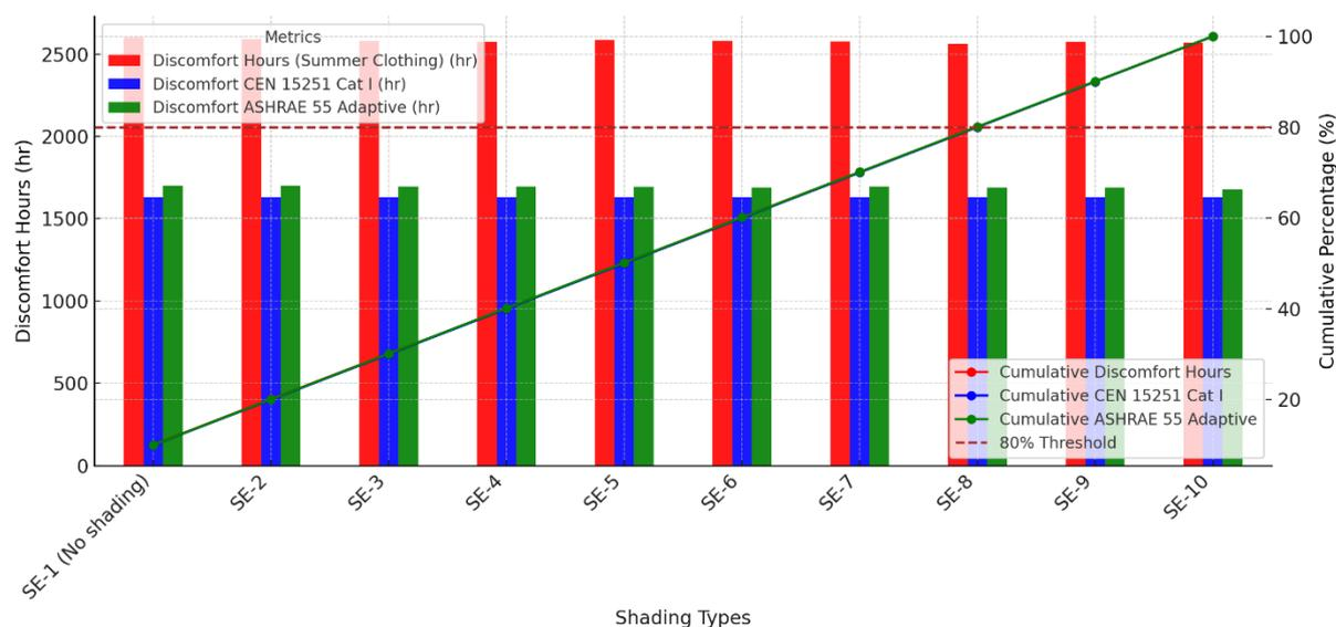
**Figure 7.** Impact of Different Shading Elements on Discomfort Hours Under Natural Ventilation (VT-1) at a Fixed 5% Window Opening Ratio
