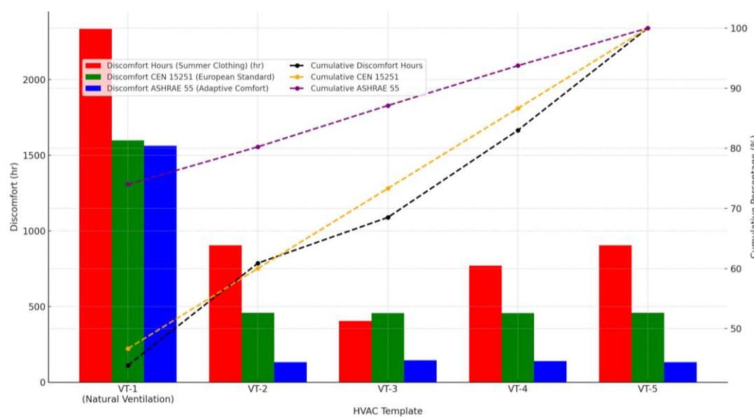
**Figure 8:** Comparison of Discomfort Hours Across HVAC Systems at 5% Window Opening Ratio and SE-1 (No Shading) Using Pareto Analysis
