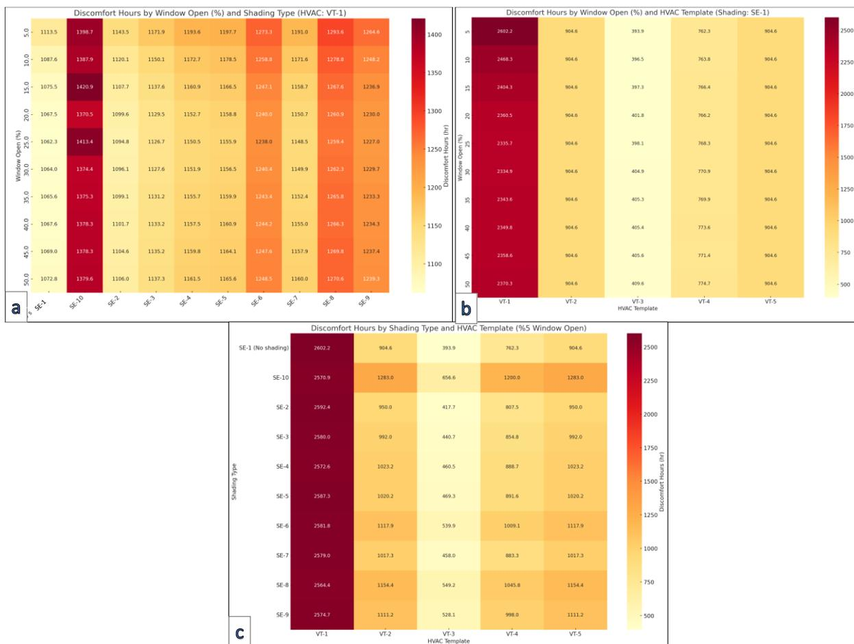
**Figure 11 (a).** Heatmap of Discomfort Hours by Window Opening Percentage (%) and Shading Type (HVAC: VT-1), **(b).** Heatmap of Discomfort Hours by Window Opening Percentage (%) and HVAC Template (Shading: SE-1), **(c).** Heatmap of Discomfort Hours by Shading Type and HVAC Template (5% Window Open)
