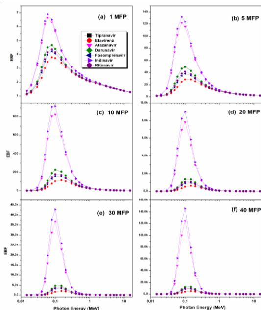
**Figure 5.** The variations in EBF with photon energy at 1, 5, 10, 20, 30, and 40 MFP for the investigated drugs.
