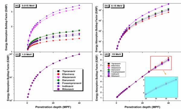
**Figure 7.** The EABF values for the investigated drugs up to 40 MFP at 0.015, 0.15, 1.5, and 15 MeV.
