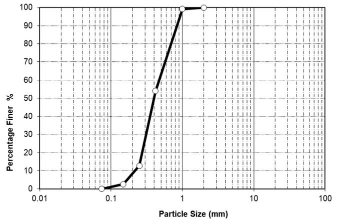
Fig. 3. Grain size distribution of sand
