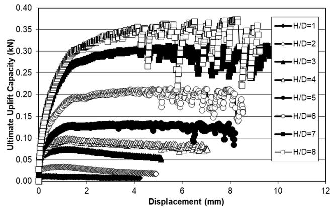
**Fig. 4.** Variations of uplift capacity with displacement for model tests ( $Dr=35\%$ )
