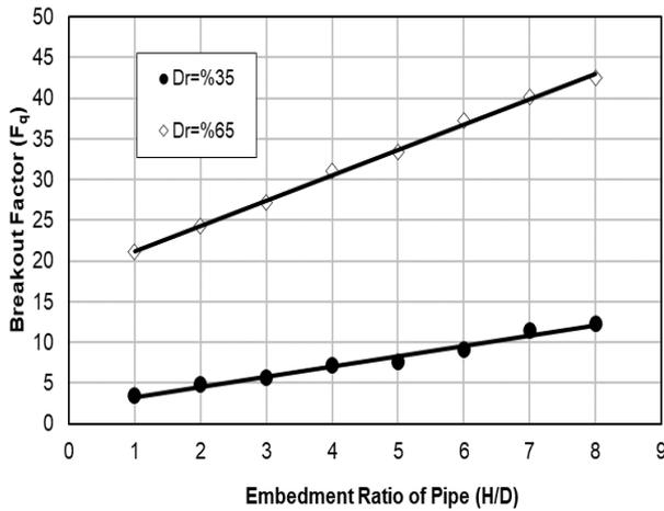
**Fig. 6.** Variations of breakout factor with embedment ratio of pipe
