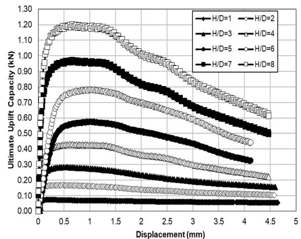
**Fig. 5.** Variations of uplift capacity with displacement for model tests ( $Dr=65\%$ )
