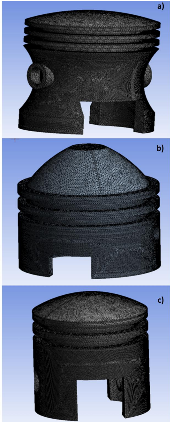
Figure 4. a) Mesh view of piston head design 1, b) piston head design 2, and c) piston head design 3
