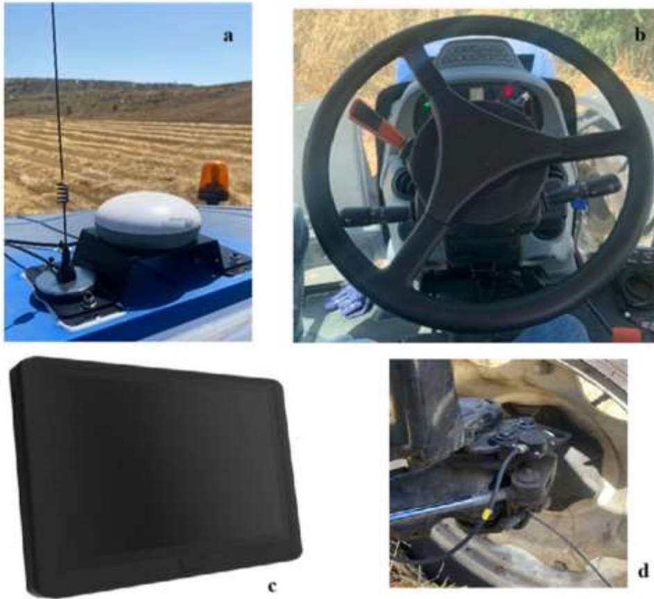
Figure 1. Automatic steering system used for trial (a: antenna, b: motorized steering wheel, c: display screen, d: angle sensor)
