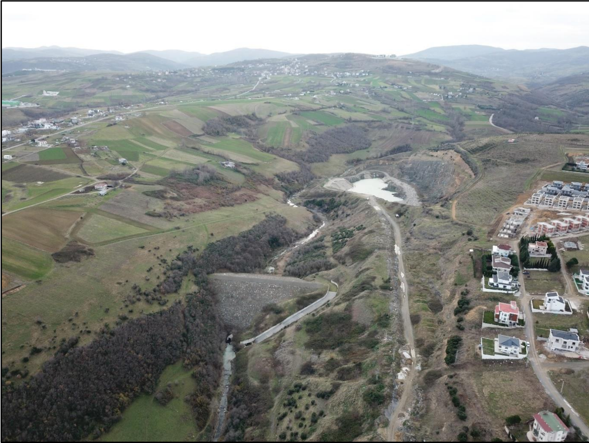
Figure 4. A flood protection barrier constructed over the river in Yenimahalle, one of the most populous neighbourhoods in Atakum, to safeguard against flooding. Residences are observed right at the edge of the stream.
