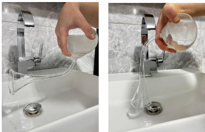
Figure 20-21. Drainage of liquid from the vase in two distinct holding positions with the spout in an closed position.
