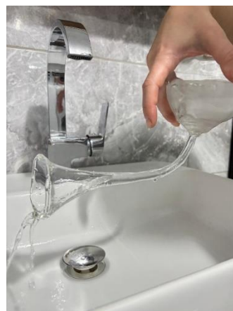
Figure 18-19. Drainage of liquid from the vase in two distinct holding positions with the spout in an open position.
