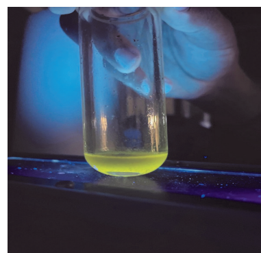
Figure 1. The physical appearance of IMQDs under UV light (365 nm).
