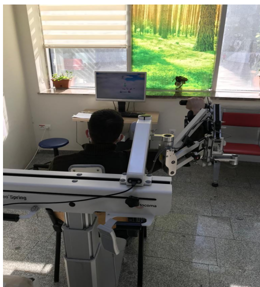
Figure 2. The Armeo Spring is an exoskeleton apparatus with an integrated spring mechanism allowing variable upper limb gravity support.
