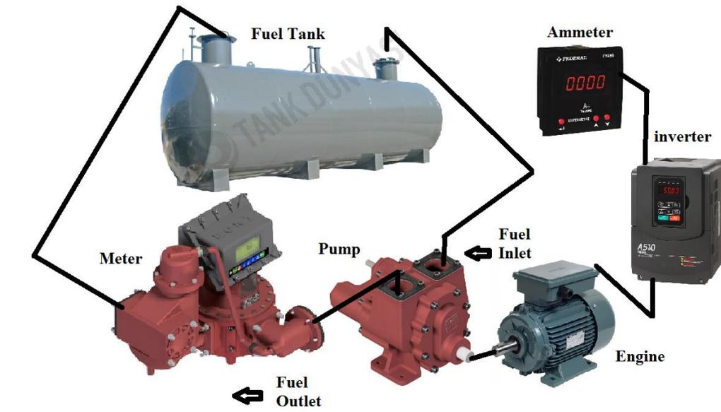
*Figure 1. Fuel transfer power consumption test setup*
