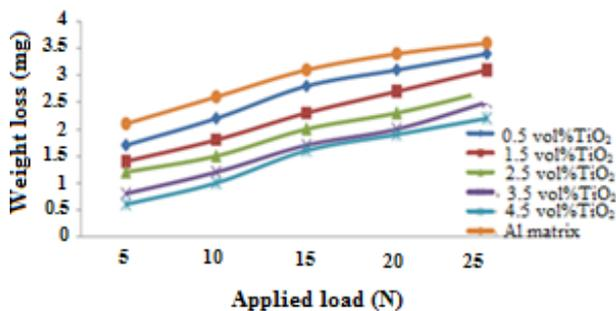
Figure 14. Effects of applied load on wear resistance [2]
