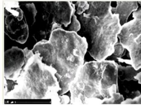
Figure 5. Morphology of Al powder milled for 12 h [13]
