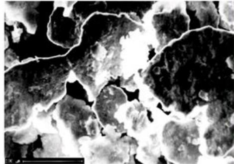
Figure 6. Morphology of Al powder milled for 18 h [13]
