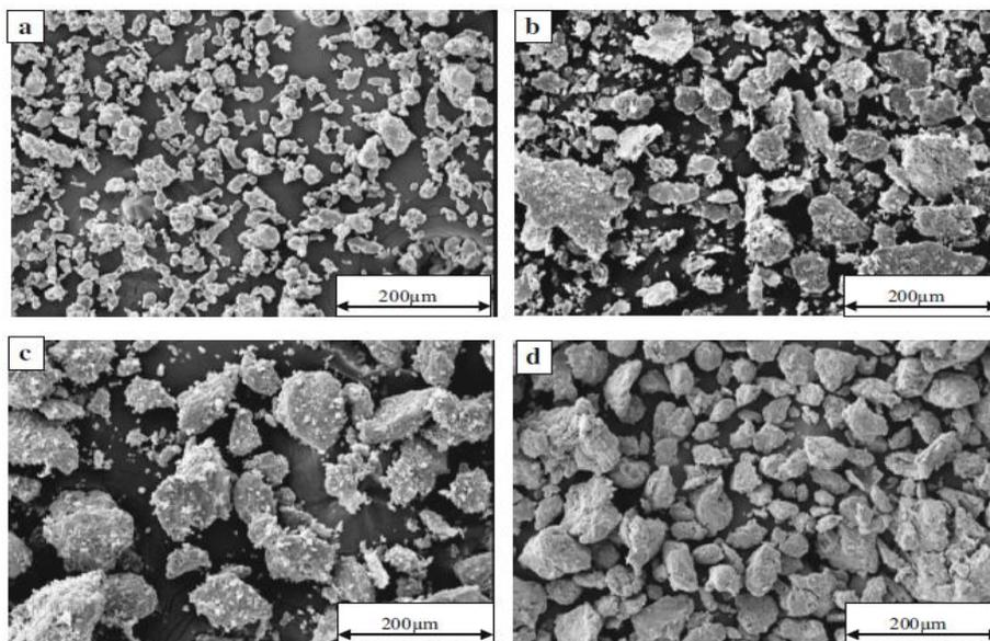
Figure 7. The evolution of morphology during mechanical milling of Al-2.5wt.%SiC nanocomposite powder milled for: (a) 2 h, (b) 15 h, (c) 20 h and (d) 25 h [14]
