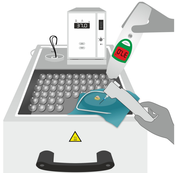
Figure 2. The experimental setup used to simulate the oral environment in this study
