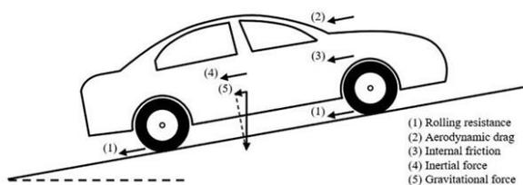
Figure 2.4 Illustration of the different factors affecting vehicle driving resistance [25]
