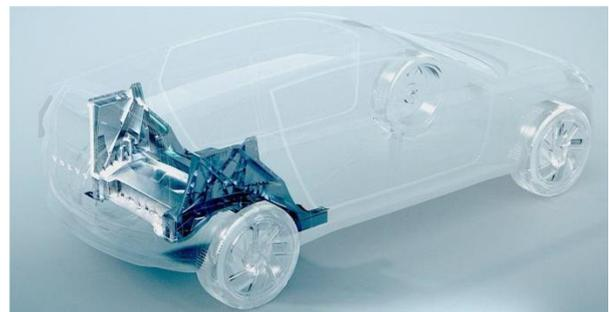
Figure 3.18 Volvo mega-casting example [58]
