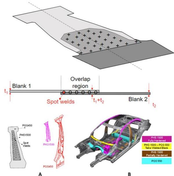
Figure 3.20 Overlapped patch sheet welding (a) and Jaguar I-Pace B-pillar (b) [70,71]
