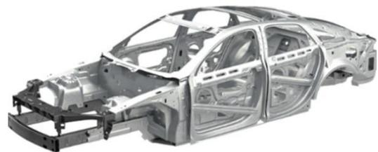
Figure 2.1 BIW design and monocoque structure [12]
