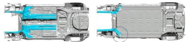
Figure 3.11 Ford Mach-E ICE-BEVs floor structure comparison [41]
