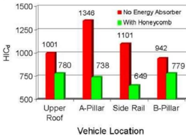
Figure 2.5 Impact absorption responses of honeycomb structures based on vehicle chassis regions [30]
