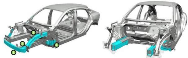
Figure 3.1 Ford Mustang Mach-E front support component modifications [41]
