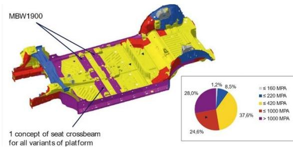
Figure 3.13 Sheets used in the Volkswagen ID.3 platform's floor structure [50]
