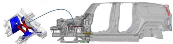
Figure 3.4 Addition of front support bracket for GM
