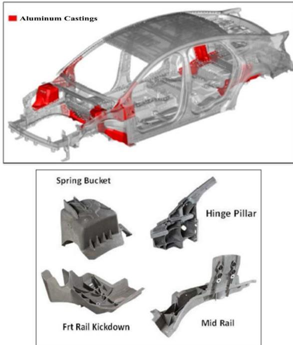
Figure 3.15 MMLV body aluminum casting parts [33]
