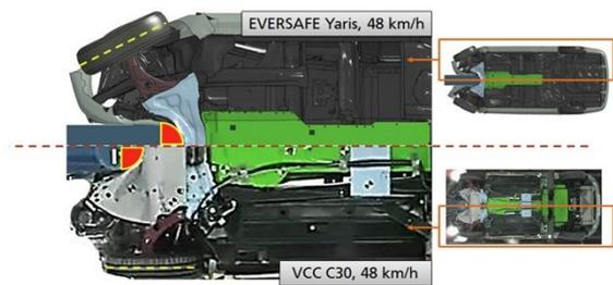
Figure 2.2 Eversafe front crash test (Top: Toyota Yaris, Bottom: Volvo C30) [16]
