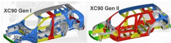
Figure 3.5 Volvo XC90 ICE B-Pillar replacement [10]
