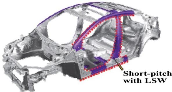
Figure 3.21 Toyota factory Lexus LSW application method [73]
