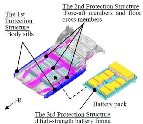
Figure 3.12 Central floor structure connections [49]
