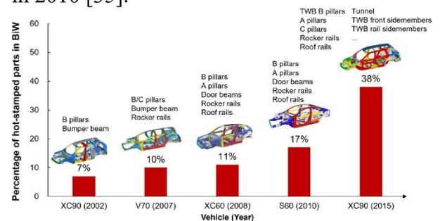
Figure 2.6 Use of hot-stamped components in Volvo [35]
