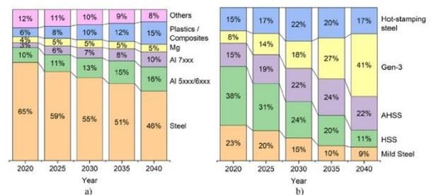
Figure 2.7 General materials used in BIW(a) and the ratio of steel materials over the years (b) [35]
