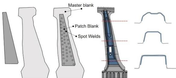
Figure 3.19 Geometries of the main blank and patch for the B-pillar: (a) before, (b) after the spot welding process, (c) after hot forming [68]
