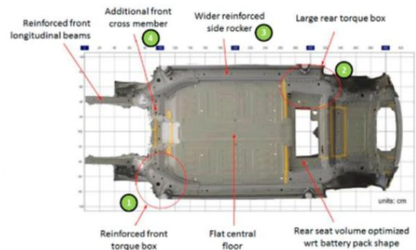
Figure 3.10 Jaguar I-Pace floor structure (Left: ICE, right: BEVs) [48]
