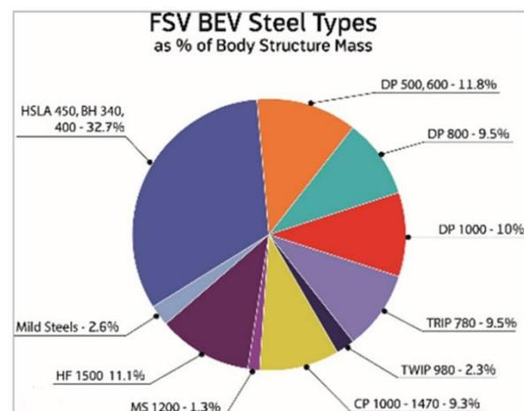
Figure 2.8 Steel types used in BEVs [38]
