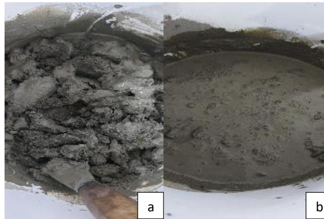
**Figure 5.** (a) Non-fluid mortar mixture, (b) Mortar mixture that becomes fluid with additive
