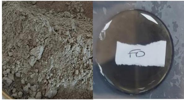
**Figure 2.** Preparation of cement in glass tablet form using the fusion method
