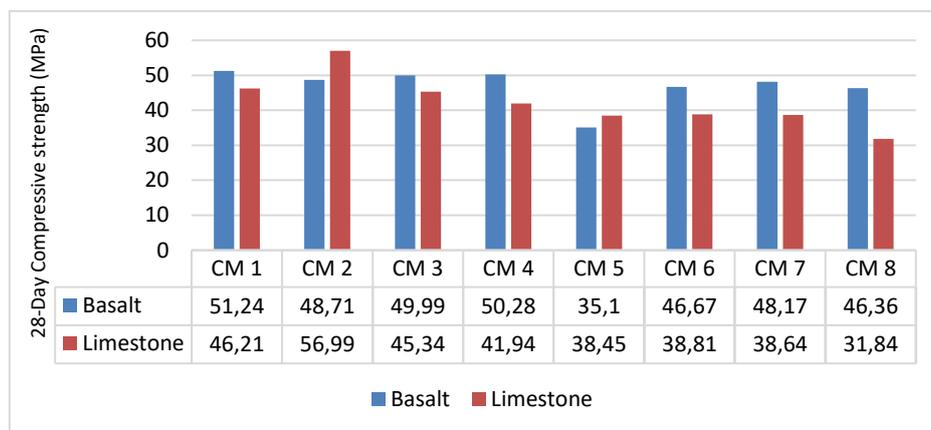
Figure. 28-day Compressive Strength Of Cement Mortars Prepared with Basalt and Limestone Aggregates
