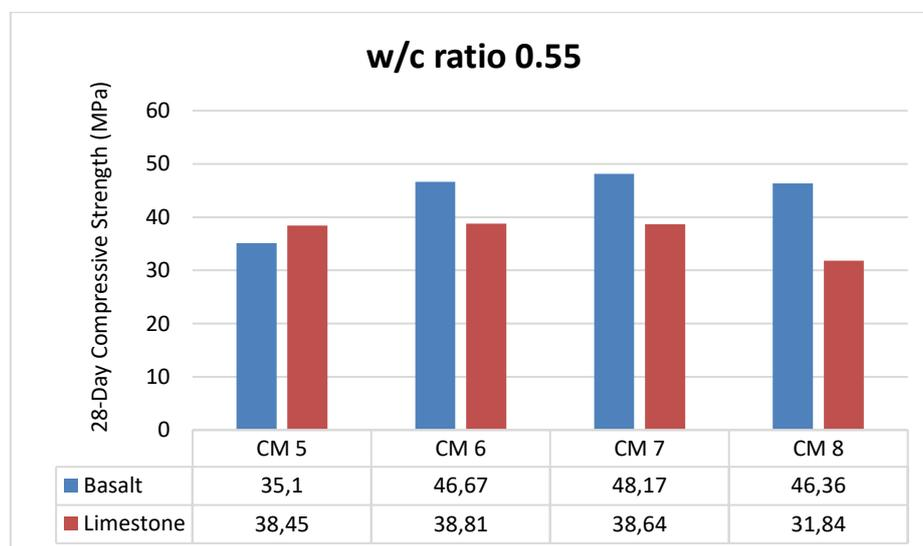
**Figure 18.** 28-day compressive strengths of mortar mixtures prepared with basalt and limestone aggregates with a w/c ratio of 0.55 and according to additive ratios
