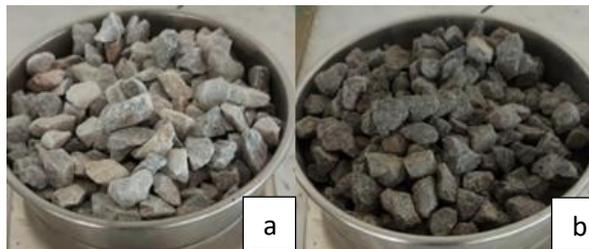
**Figure 3.** Limestone (a) and basalt (b) aggregates used in the study
