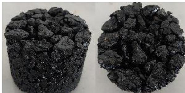
**Figure 12.** Porous asphalt specimens with limestone aggregate compacted to 35 impacts on both surfaces
