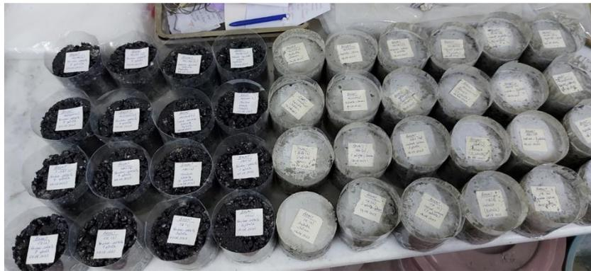
Figure 13. Porous asphalt and semi-rigid mix specimens
