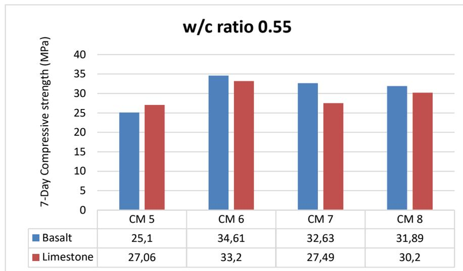
**Figure 17.** 7-day compressive strengths of mortar mixtures prepared with basalt and limestone aggregates with a w/c ratio of 0.55 and according to additive ratios
