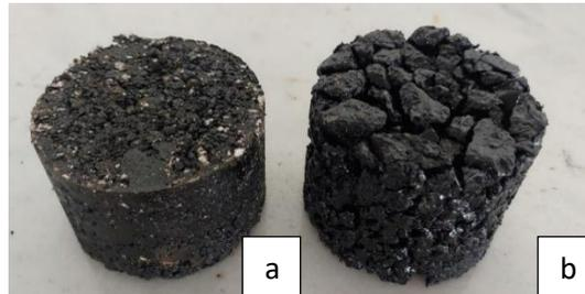
**Figure 10.** (a) Conventional asphalt mix and (b) Porous asphalt mix marshall specimens
