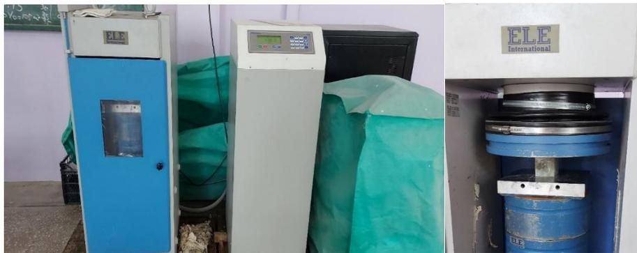
**Figure 8.** Fully automated press machine
