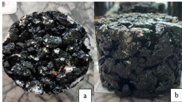
**Figure 11.** (a) Crushing of limestone mixed specimen with 50 strokes on both surfaces and (b) specimen without sufficient void ratio
