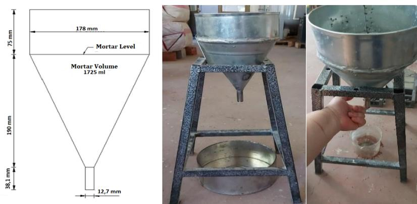
**Figure 6.** Flow cone used to determine the fluidity of cement mortar
