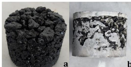
**Figure 1.** (a) Low air void content of porous asphalt mix and (b) insufficient cement injection
