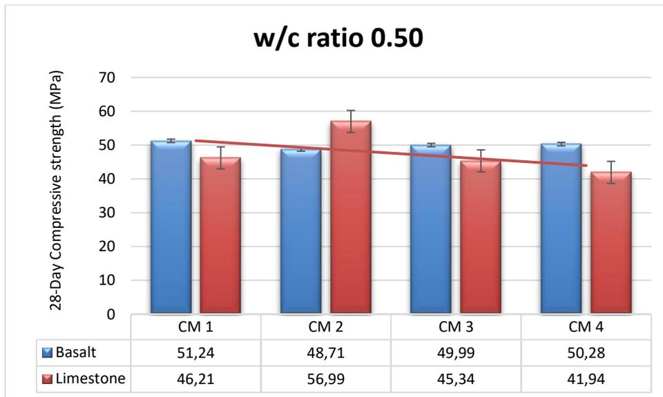
**Figure 16.** 28-day compressive strengths of mortar mixtures prepared with basalt and limestone aggregates with a w/c ratio of 0.50 and according to additive ratios
