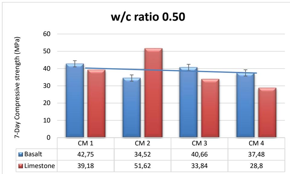
**Figure 15.** 7-day compressive strengths of mortar mixtures prepared with basalt and limestone aggregates with a w/c ratio of 0.50 and according to additive ratios
