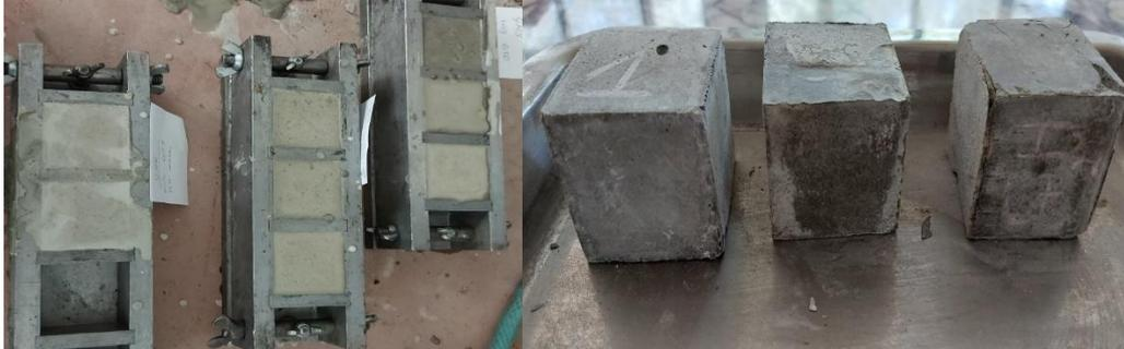
**Figure 7.** Molds and samples used for the compressive strength of cement mortar
