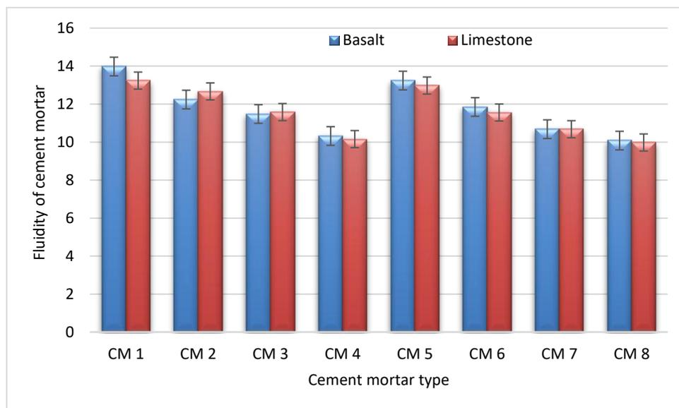
Figure 14. Fluidity times of mortar mixtures prepared with basalt and limestone aggregate
