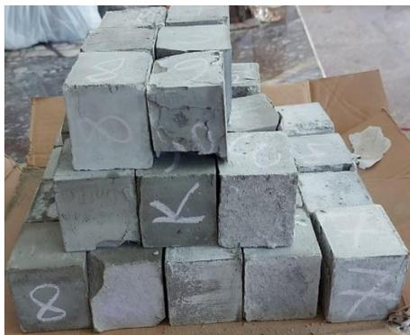
**Figure 9.** Samples of cement mortar after the applied compressive strength test
