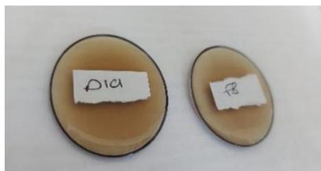
**Figure 4.** Conversion of basalt and limestone aggregates into glass tablet form
