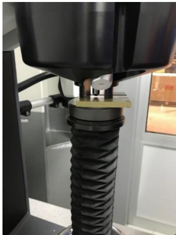
Figure 7. Sample view connected to the device for hardness testing
