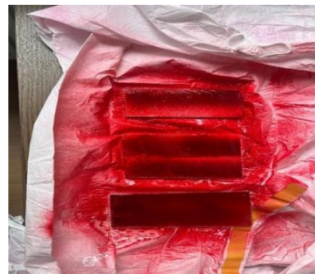
Figure 15. Specimens following the application of red penetrant during liquid penetrant testing [icmatse2024]
