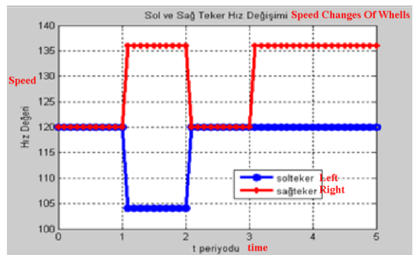
Fig.10. Velocity change of right (red) and left (blue) front wheels at different time step
