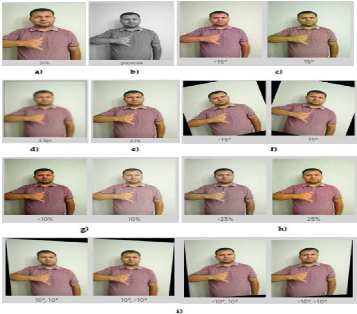
Figure 2. a) Modification of size and position, b) Conversion to grayscale, c) Slope adjustment, d) Application of blur, e) Rotation variability, f) Introduction of noise, g) Adjustment of brightness, h) Alteration of colour intensity, i) Perspective distortion.
