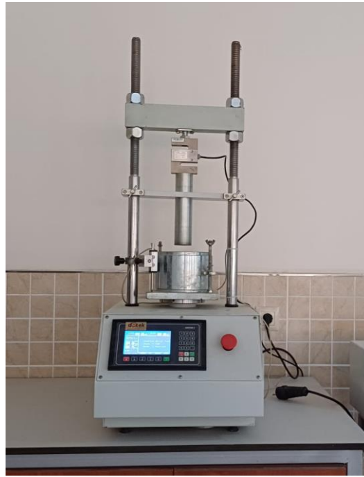
Figure 3. CBR test setup
