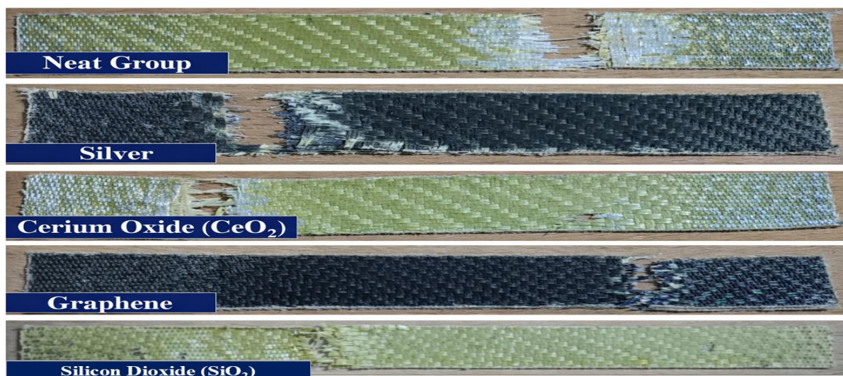
Figure 5. Damage images of tensile test specimens of nanoparticle doped composites
