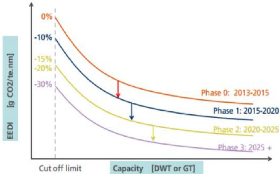
**Figure 10.** Concept of Required EEDI, reduction factor, cut off limits and EEDI phases [32]
