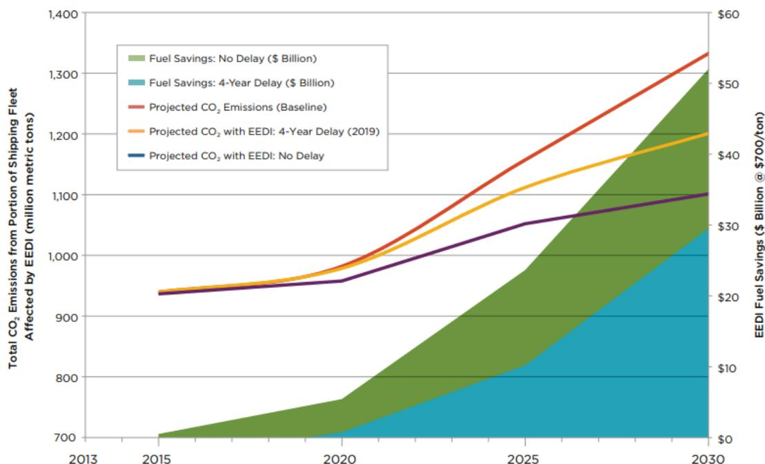
**Figure 2.** Projected CO<sub>2</sub> emissions and cost savings through 2030 from the shipping fleet affected by EEDI Regulation. IMO Scenario A2, with and without proposed 4-year delay [19]
