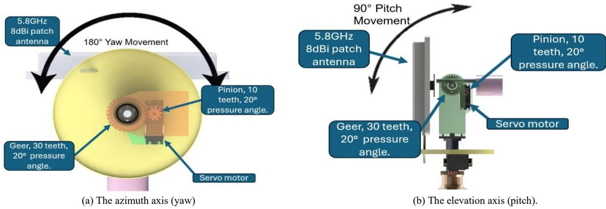
Figure 6. Movement of every axis: (a) azimuth axis (yaw); (b) elevation axis (pitch)
