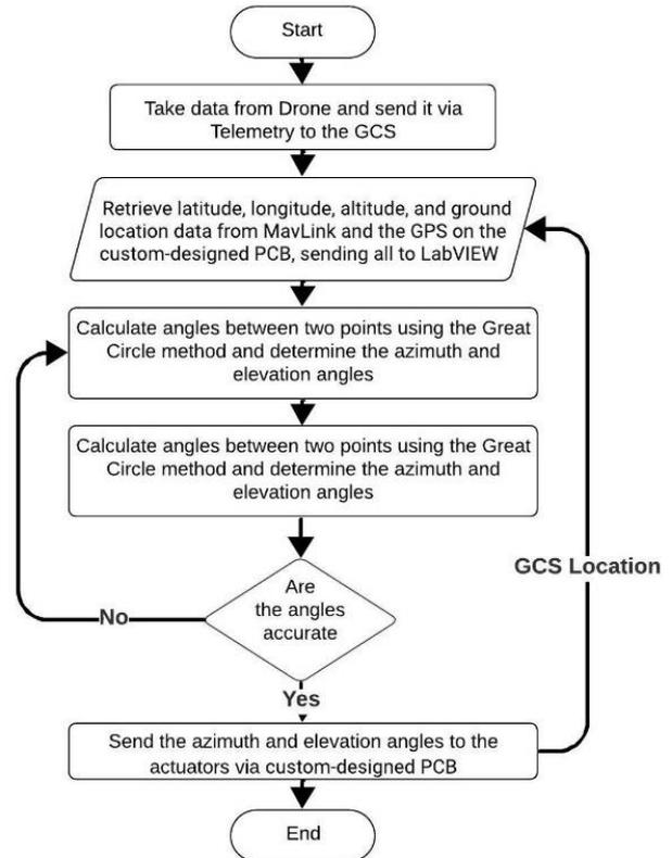
**Figure 2.** The flowchart of the proposed antenna tracking conceptual in this study
