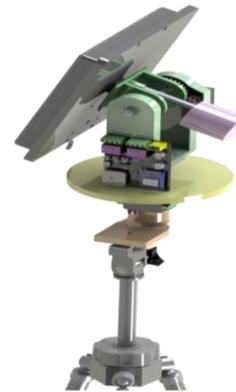
**Figure 5.** 3D design of antenna tracker
