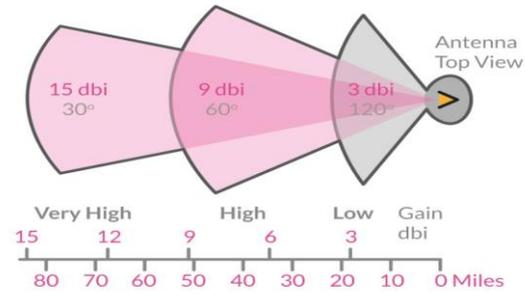
Figure 1. The Impact of Gain on Antenna Range [3]
