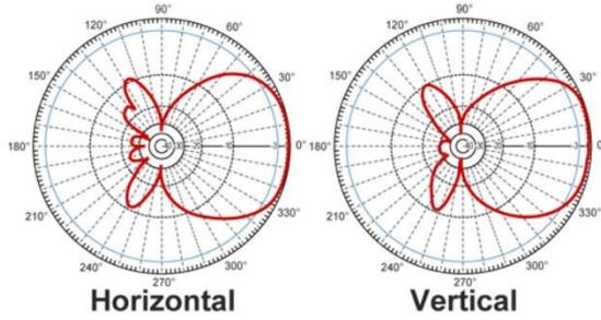
Figure 8. Radiation pattern for 8 dBi patch antenna [7]
