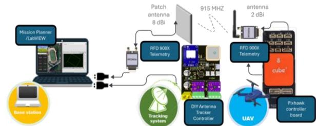
Figure 7. Telemetry configuration
