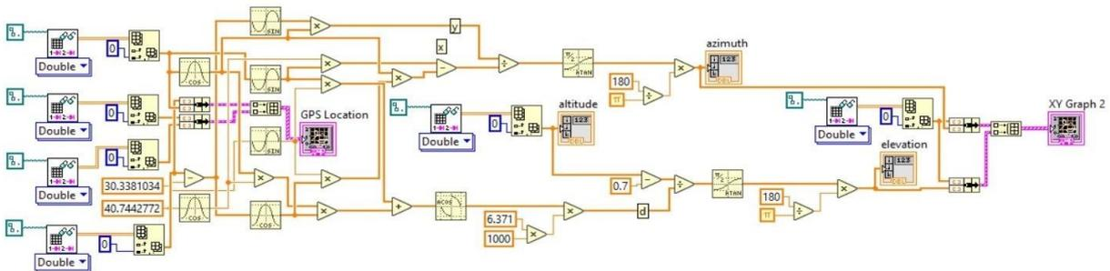
Figure 9. The LabVIEW Block diagram of mathematical calculations
