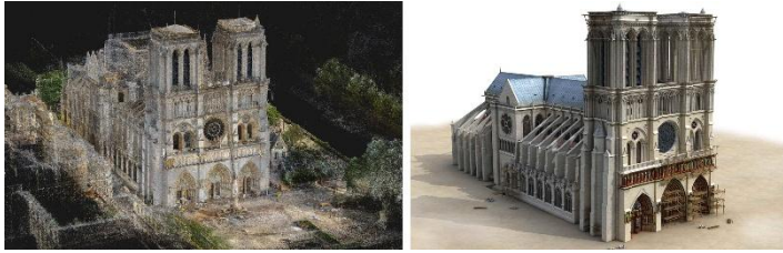
Figure 18. 3D laser scanning point cloud (left) and BIM model (right) for Notre Dame Cathedral Restoration (URL-1)
