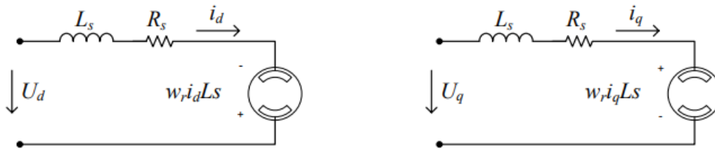
Figure 3. Equivalent circuit of the electric motor
