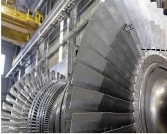
Figure 4. The turbine blade that has completed its working life, and the areas from which samples are taken
