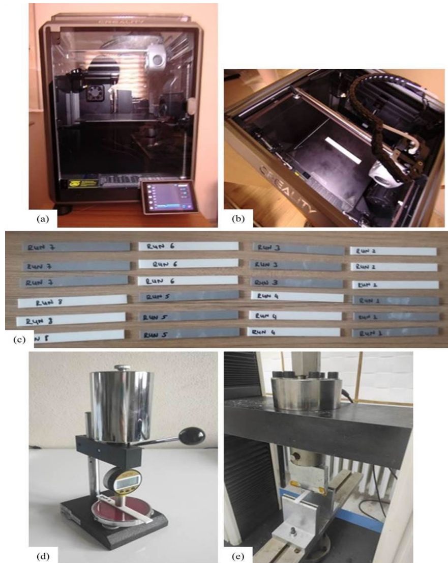
Figure 2. 3D printer used for specimen production (a), specimen fabrication (b), test specimens (c), shore D hardness gauge and measurement operation (d) and three-point bending test device and bending operation (e).
