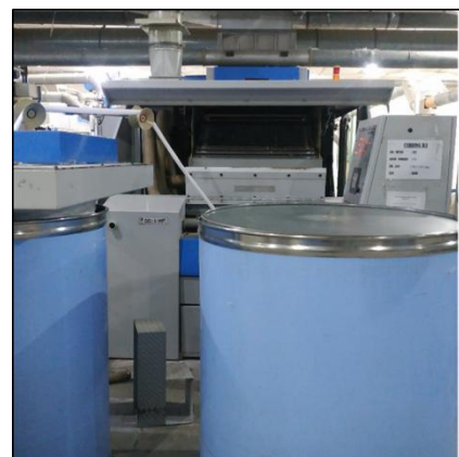
Figure 1. Photograph of the Ming Cheng carding machine (B2/B3) used in the study, showing the sliver drums and operator interface in the production facility.
