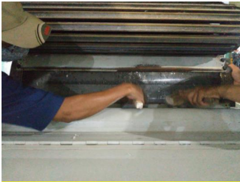
Figure 5. Photograph showing the manual cleaning process of the wire cylinder using a lint-free cloth and soft-bristle brush, as performed during scheduled maintenance.
