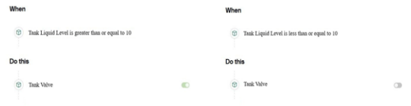
Figure 14. Tank liquid level trigger mechanism.
