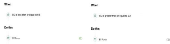
Figure 12. EC trigger mechanism.
