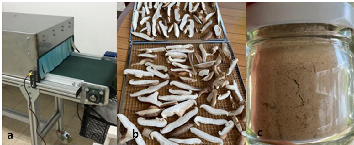
Figure 1. Application to the mushroom samples: (a) UV-B conveyor system, (b) Sliced and panned mushroom samples, (c) dried and powdered mushroom sample
