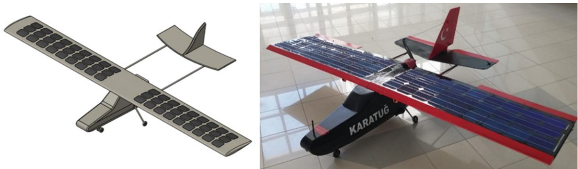
Figure. Aircraft featuring solar panel cells on its wings – illustration and actual
