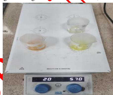
Figure 1. Preparation of coating solutions (Magnetic stirrer).
